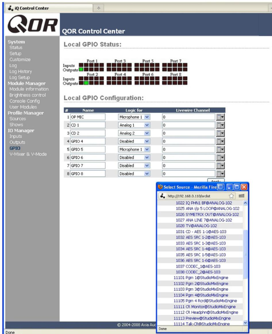
Figura 2-8: GPIO Configuration
